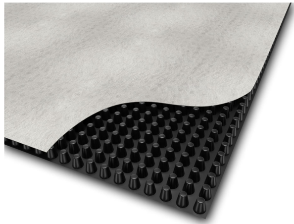
Fig. 1: Deckdrain geocomposite with cusped drainage core and integral filter geotextile. Deckdrain is installed with the textile facing upwards, as shown above
