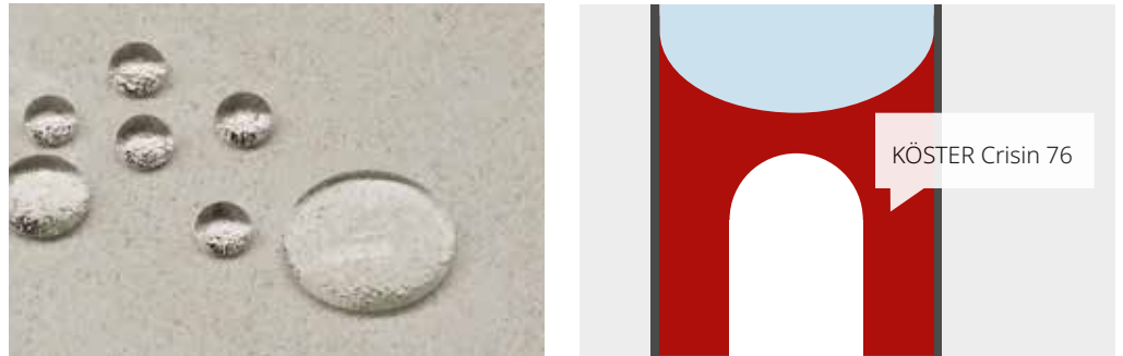
Hydrophobizing: Making the building material water repellent
