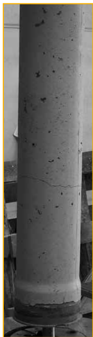
first crack (150 N/mm 2 )
